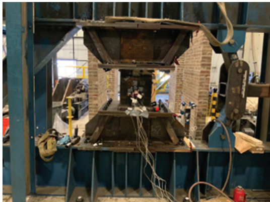
Fig. 8. Test setup of shear component specimen.
